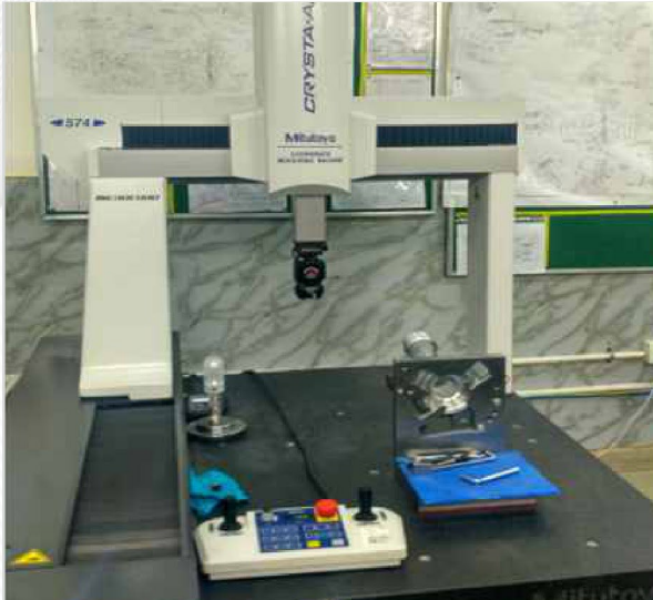
Full Tessa CNC co-ordinate measuring machine (CMM)
