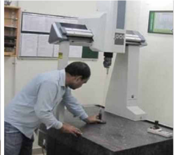
Mitutoyo CNC co-ordinate measuring machine (CMM)
